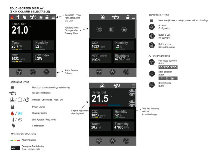
The touchscreen is divided to three different main elements; Status Bar, Measurement/Setpoint Display Locations and Buttons (accessible on the Action Bar on the bottom or via the Menu Icon on the top).
