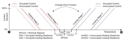
The multi-stage temperature control loop can be configured to control built-in temperature, Universal Input 1 temperature/voltage, Universal Input 2 Temperature/voltage, or network value (network temperature).
