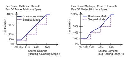
Fan Speed Settings : Default. Except Fan Off Mode Fan Off Mode: Off (Fan Off at 0% Demand)
