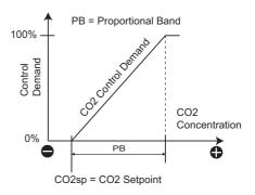
Cooling Stage temperature control and CO2 control. This can be achieved using so called 'Maximum VAV' logic (set output to *Maximum VAV*).
