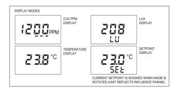
Note: The backlight is permanently on if activated. At 50% intensity the backlight lifetime is approx 10,000 hours. After this time the LCD module needs replacing if backlight is required. The display continues to operate without backlight.
