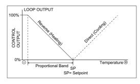
modulate to 100%. When the temperature is the amount of the Proportional Band below the setpoint the loop output is 100%. In the Direct Control mode the output modulates in reverse. The configuration is done via the configuration parameters.
