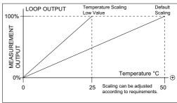
Furthermore the temperature measurement reading can be adjusted on site using the Single Point Calibration field.
