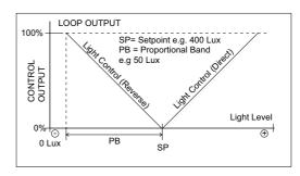
the setpoint the loop output is 100%. In the Direct Control mode the output modulates in reverse. The configuration is done via the configuration parameters.
