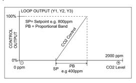
the setpoint the loop output is 100%. The configuration is done via the configuration parameters. The CO2 control loop can also be configured to operate as Proportional + Integral control by changing the Integral Action Time from 0 to a required value.
