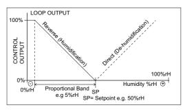
starts to modulate to 100%. When the humidity is the amount of the Proportional Band below the setpoint the loop output is 100%. In the Direct Control mode the output modulates in reverse. The configuration is done via the configuration parameters (or over Modbus network).
