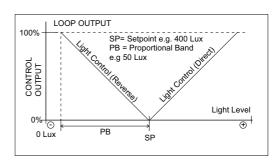
the setpoint the loop output is 100%.In the Direct Control mode the output modulates in reverse. The configuration is done via the configuration parameters (or over the Modbus network).
