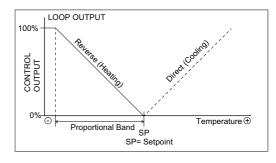
modulate to 100%. When the temperature is the amount of the Proportional Band below the setpoint the loop output is 100%. In the Direct Control mode the output modulates in reverse. The configuration is done via the configuration parameters (or over the Modbus network).
