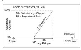
Proportional Band above the setpoint, the loop output is 100%. The configuration is done via the configuration parameters (or over the Modbus network). The CO2 control loop can also be configured to operate as Proportional + Integral control by changing the Integral Action Time from 0 to a required value.
