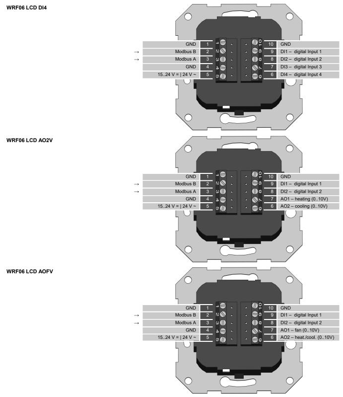
BUS connection type DO2R/DO2T/OVR/OVT  $\rightarrow$  Terminal 2 and 3 on the basic unit.
