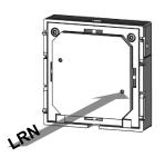
After delivery the room operating unit might be in default shipping mode, in this case press the learn button (<1 second) at the rear of the device [Signal telegramm will be send. SIG ->  $0x0F \parallel$  shipping mode deacticvated].
