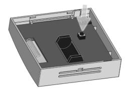
After delivery the room operating unit might be in default shipping mode, in this case press the learn button (<1 second) at the rear of the device [Signal telegramm will be send. SIG -> 0x0F // shipping mode deacticvated].
