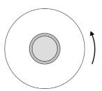
To access the Learn button, turn the sensor cover counterclockwise and remove the cover.
