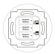
The SR-MDS BAT is battery powered, a wired connection is not necessary. Remove the cover from the backside of the device to insert/exchange the batteries.
