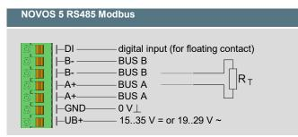
Don't forget the BUS termination (120  $\Omega$ ) at the last device of the line!
