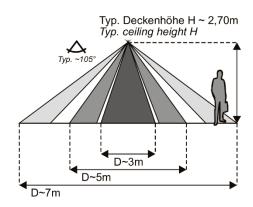
This sensor detects changes in infrared radiation that occur when a person (or object) moves whose temperature is different from the environment.
