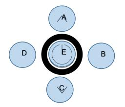
Menu navigation on the touch-surface is performed by pressing the buttons "up" (A), "down" (C), "left" (D), "right" (B) or the power button. Choose the desired parameter and press "right" (B) to open up the submenu. The menu will default after 30 seconds if no button is pressed. To exit the menu select the header line and press "left" (D).
