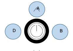
The configuration menu is called up by simultaneously pressing the buttons "up" (A), "left" (D) and "right" (B) for at least 3 seconds.
