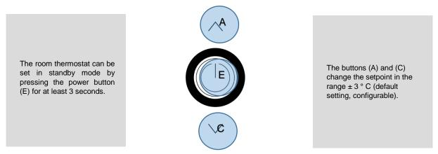
With power-button (E), the device can be set in standby mode by pressing the button (if keycard-switch is NOT used). If the button is used as a occupancy button, the button must be pressed for at least 3s, in all other cases, a short actuation is sufficient. In standby mode, the display and all outputs are switched off (controller deactivated). The frost and heat protection monitoring remains active. **Modbus registers can still be read (e.g. room temperature).**
