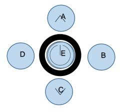
Menu navigation on the touch-surface is performed by pressing the buttons "up" (A), "down" (C), "left" (D), "right" (B) or the power button. Choose the desired parameter and press "right" (B) to open up the submenu. The menu will default after 30 seconds if no button is pressed. To exit the menu select the header line and press "left" (D).
