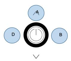
The configuration menu is called up by simultaneously pressing the buttons "up" (A), "left" (D) and "right" (B) for at least 3 seconds.
