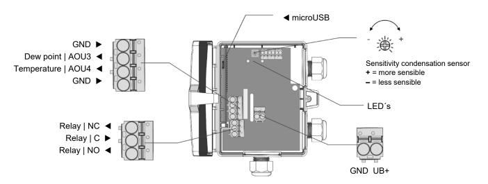
The relay is energized in the operating state (relays NO and C connected). Upon dew permeation or when the operating voltage is switched-off, the relay falls off.
