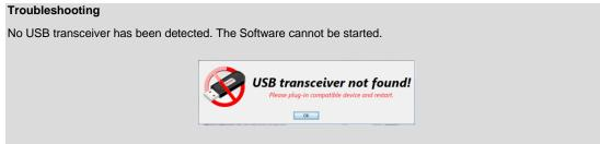
In this case please check in your device manager whether the USB transceiver has been detected properly and the driver is installed. If the driver is missing, you may download the appropriate driver for your system from <a href="http://www.ftdichip.com/Drivers/VCP.htm">http://www.ftdichip.com/Drivers/VCP.htm</a>.
